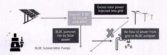
As shown above, DC power from solar panels is passed through DC-DC circuit and Maximum Power Point Tracker (MPPT) to operate the BLDC submersible pump. Excess solar power is converted to AC power using Inverter and is injected into the grid. The benefits for famers include the following:
